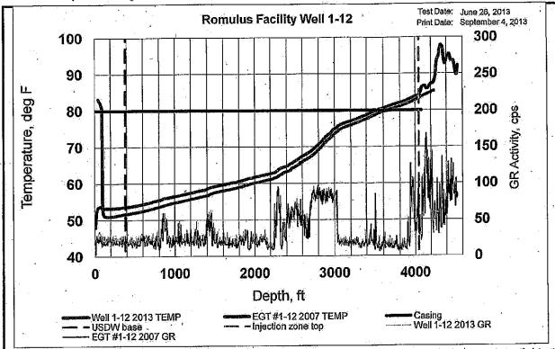
The 2013 test mirrors the 2007 test very well. There appears to be a sudden drop in temperature right at the start of the test, this is most likely caused by the hight temperature outside on the testing day. The other major difference is in the injection zone. In the 2013 test the curve remains constant after entering the injection zone. For the 2007 test there was a rise in temperature after entering the injection zone.
